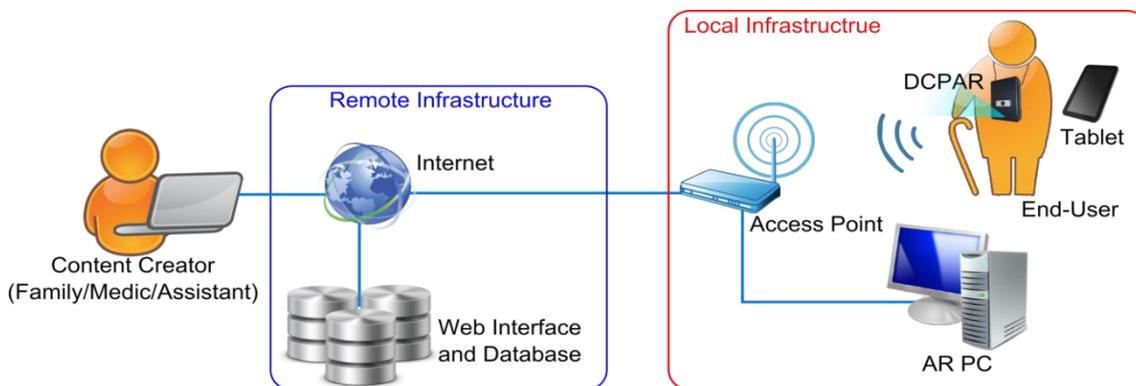
Figure 2 . Design of the experimental Assisted Living system.
